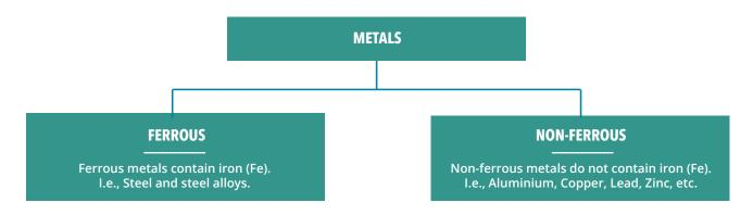
Steel, an iron alloy containing less than 2% of carbon (highly ductile), is by far the most used metal in the world. Followed by aluminium and copper, and other non-ferrous metals such as lead, zinc, nickel, titanium, cobalt, chromium and specialty and precious metals.
