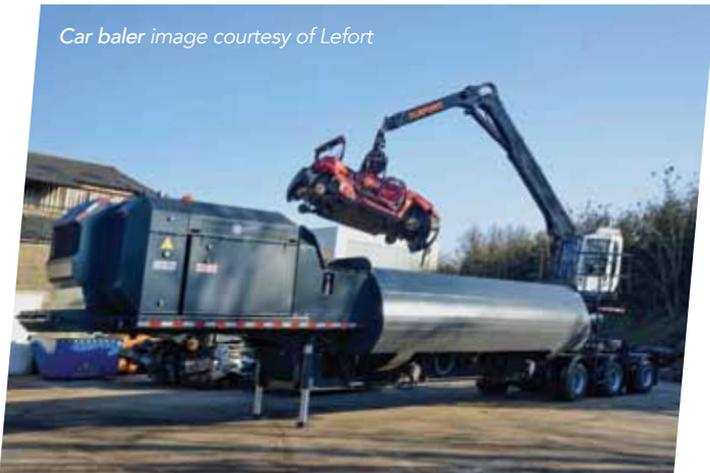
If the metal recycler doesn't have the means to shred or separate metals, they might use a baler, that can crush, cut and bale metal enabling a more compact size for transportation.
